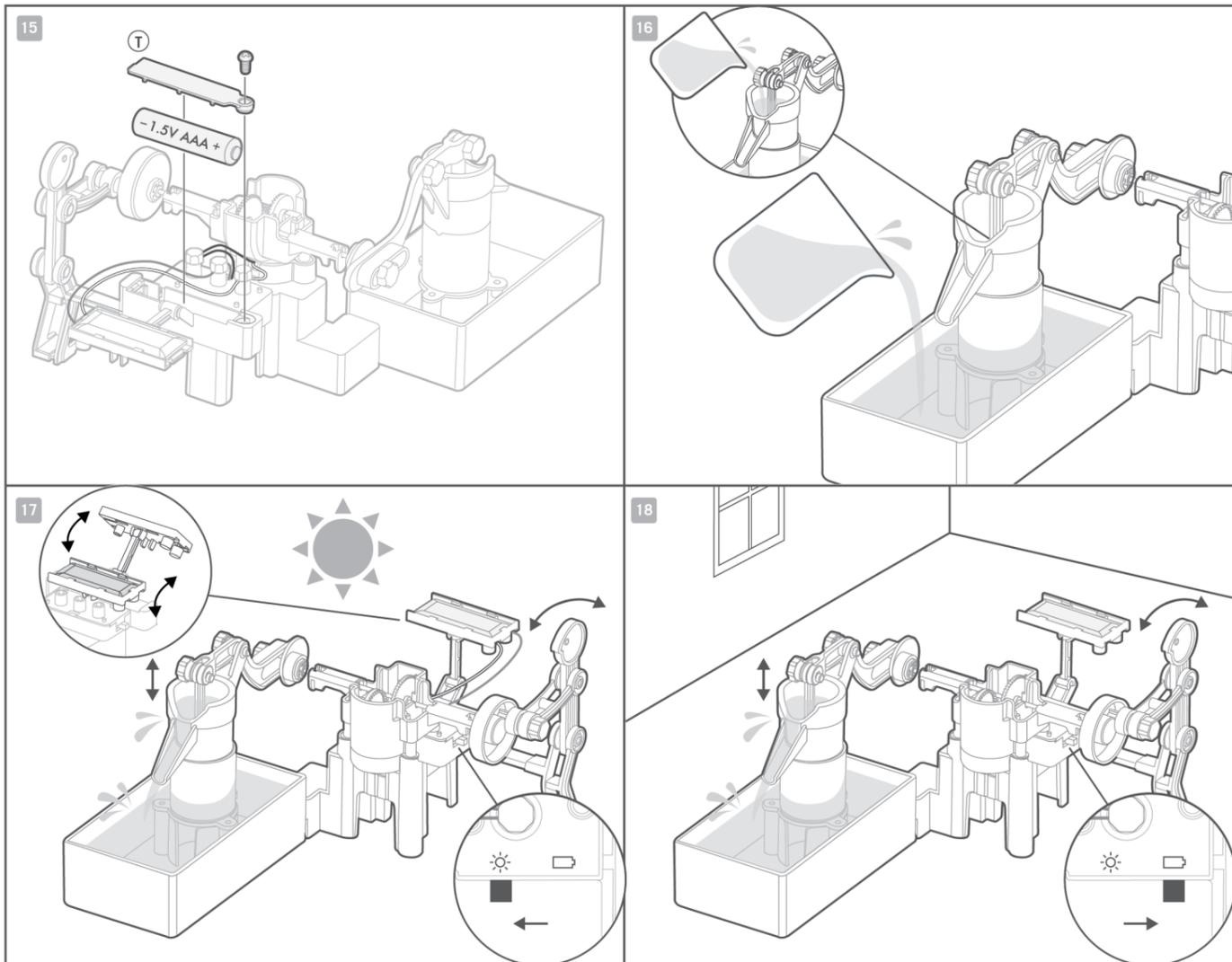
15. Match up the polarities of the battery with the markings on the case before you put it in. Secure with the battery cover. Your water pump is now complete!
