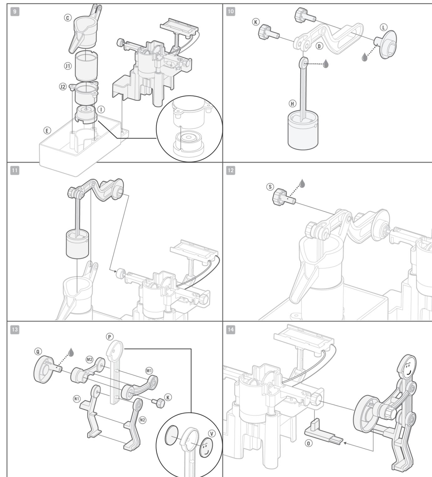
9. Align each notch with the small cutout on parts (C, I, J1, and J2) as shown in the small diagram. Insert (J2)'s 3 joints into the holes on the pump base to secure the completed cylinder in place. Water will flow smoothly through the system only if the pieces are connected correctly. Finally, connect the main frame to the pump base as shown.
